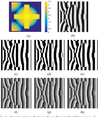
Fig. 4. Experimental results I: (a) object, (b) normalized fringe image  $I_{i,j}$ , (c) true signs  $s_{i,j} = \text{sgn}(\phi_{i,j}^W)$  (to be estimated), (d) signs estimated by [12], (e) signs estimated by the proposed branch cut, (f) true wrapped phase  $\phi_{i,j}^w$ , (g) wrapped phase based on (d), and (h) wrapped phase based on (e).
