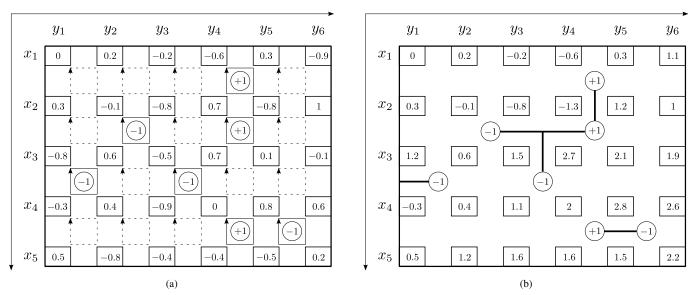
Fig. 1. Illustration of the idea of Goldstein's branch cut [20] for 2D phase unwrapping: (a) detection of every closed loop having a nonzero residue  $r_{i,j} = \pm 1$  in (7) from given normalized wrapped phase  $\phi_{i,j}^W/\pi$  (i = 1, 2, ..., 5 and j = 1, 2, ..., 6) and (b) construction of branches and the corresponding normalize unwrapped phase  $\phi_{i,j}/\pi$  (i = 1, 2, ..., 5 and j = 1, 2, ..., 6).
