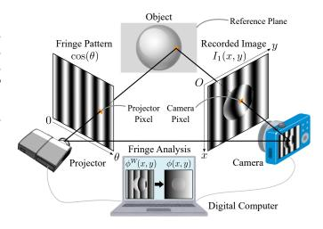
Fig. 3. Typical fringe projection profilometry system.
