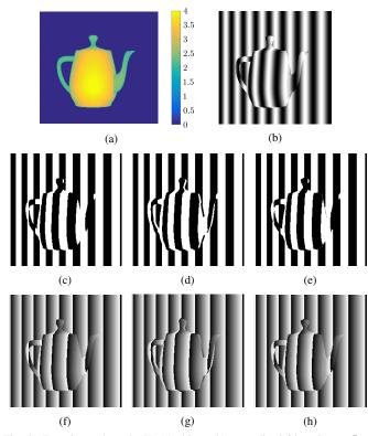
Fig. 5. Experimental results II: (a) object, (b) normalized fringe image  $I_{i,j}$ , (c) true signs  $s_{i,j} = \text{sgn}(\phi_{i,j}^W)$  (to be estimated), (d) signs estimated by [12], (e) signs estimated by the proposed branch cut, (f) true wrapped phase  $\phi_{i,j}^w$ , (g) wrapped phase based on (d), and (h) wrapped phase based on (e).
