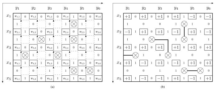
Fig. 2. Illustration of the idea of the proposed branch cut type sign estimator: (a) detection of every closed loop satisfying (12) by using the locally ideal sign changes  $c_{i,j}^{h,\min}$  and  $c_{i,j}^{h,\min}$  computed from  $v_{i,j}$  (i = 1, 2, ..., 5 and j = 1, 2, ..., 6) and (b) constructions of branches, sign changes  $c_{i,j}^{h}$  and  $c_{i,j}^{v}$ , and the corresponding signs  $s_{i,j}$  (i = 1, 2, ..., 5 and j = 1, 2, ..., 6).
